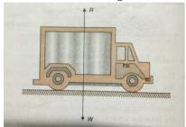
Here, the weight of the truck W is balanced by the reaction R of the ground on the truck. But the frictional force due to the ground is much more than the force of push. Therefore, the truck does not move.
